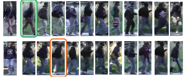
Figure 6: Top ranked images selected by our GCT algorithm. The first column are two probe images, and the following are the top ranked gallery images of each probe obtained by GCT. Images marked by green/orange bounding boxes in each row are the ground-truth matches of each probe.
